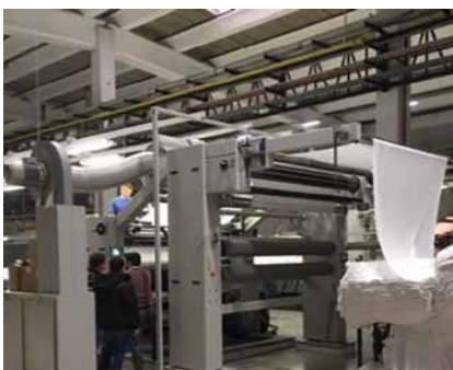
Segmented roller guider system SWA9511 on rotary printing machine infeed
