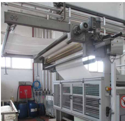
Segmented roller guider system SWS9611 in front of padder
