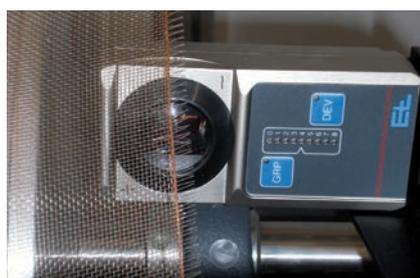
Infrared edge sensor FR 52 for mesh fabric acquisition
