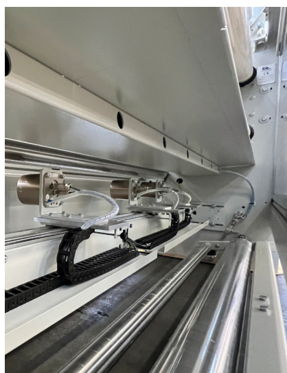
Smart cameras inspect the web straightener
