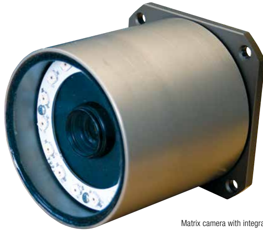
Matrix camera with integrated infrared LED flash
