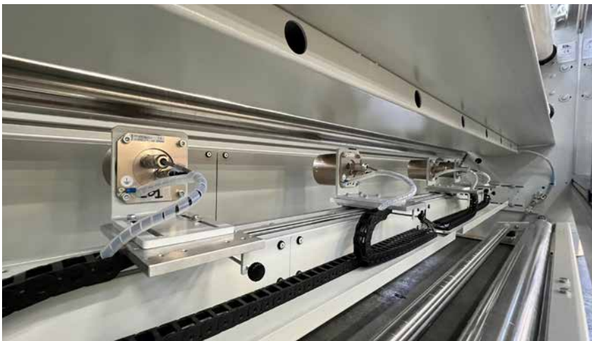
Smart cameras inspect the weft straightener
