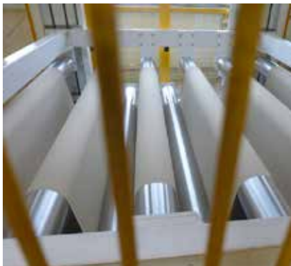
Roller accumulator, capacity 30 m, comb version
