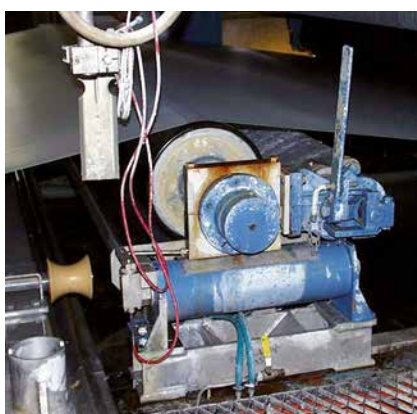
Electromechanical edge sensor SH 8902 U (optional ceramic plate) with sensor stand ST 7005
