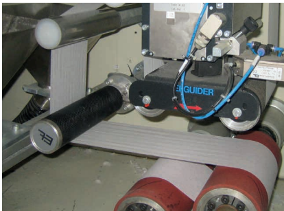
Sensorwalze PD 40 in Babywindelmaschine
